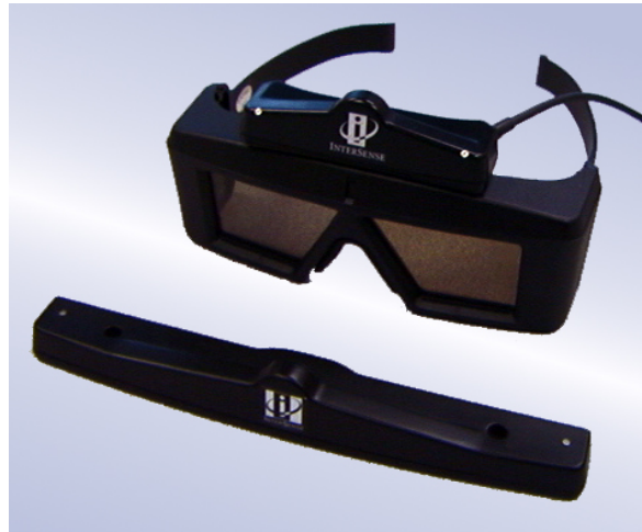
Figure 5 – MiniTrax Head Tracker on stereo glasses and the High Accuracy Head Tracker
