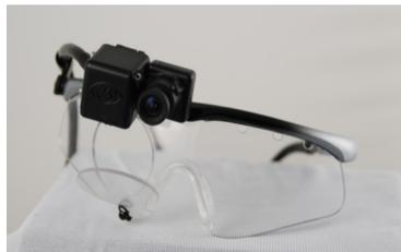
Mobile Eye-XG with Real Time wireless data transmission.
